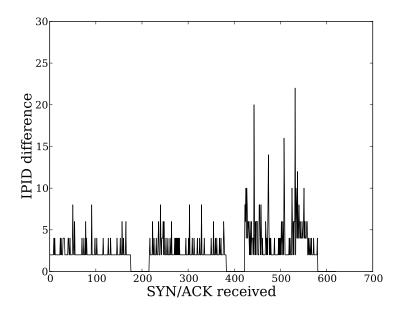
Figure 4.2: Example IPID difference time series' for three separate experiments that lead to detection of the **Server-to-client-dropped** case. Note the high amount of noise in the third experiment. Our ARMA modeling is able to detect this case correctly even in the presence of such high noise.
