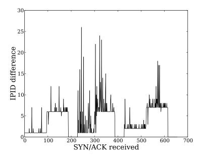
Figure 4.3: Example IPID difference time series' for three separate experiments that lead to detection of the **No-packets-dropped** case. Note the high amount of noise in the second experiment. Our ARMA modeling is able to detect this case correctly even in the presence of such high noise.
