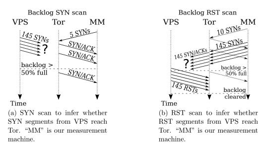
Figure 5.3: The two types of backlog scans we employ. The purpose of these scans is to verify if 1) SYN segments from China reach a Tor relay and if 2) RST segments from China reach a Tor relay.
