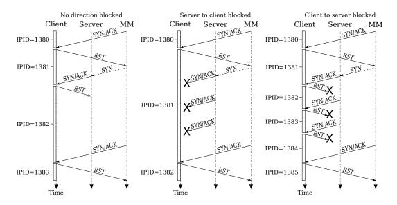
Figure 4.1: Three different cases that our method can detect. MM is the measurement machine.
