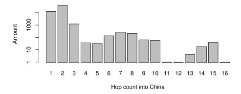
Figure 5.7: The amount of hops (log scale) in China, our filtered traceroutes could traverse. For example, a hop count of five means that a traceroute could successfully reach the fifth router inside China.
