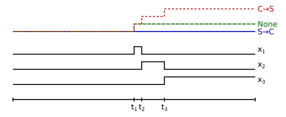
Figure 4.5: For a server that retransmits r-1 SYN/ACK's, each case can be expressed as the linear combination of regressors  $x_1, \ldots, x_r$ ; shown is when r=3 with SYN/ACK transmissions responding to the first spoofed SYN occurring at  $t_1, t_2$ , and  $t_3$ . C $\rightarrow$ S indicates client-to-server, and S $\rightarrow$ C indicates server-to-client.
